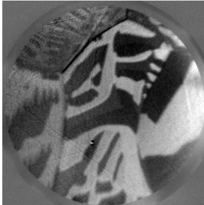
Fig. 6 Demonstration of the spin contrast on a polycrystalline iron sample in real space mode (FOV 130 \mu\text{m} ).
