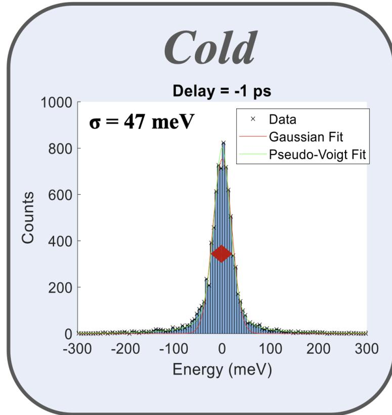
The spectrum from a cold target contains around  $\sim 10,000$  photons and was collected at 10 Hz. It is well fit by a Voigt profile with a FWHM of 47 meV, close to the theoretical instrument function
