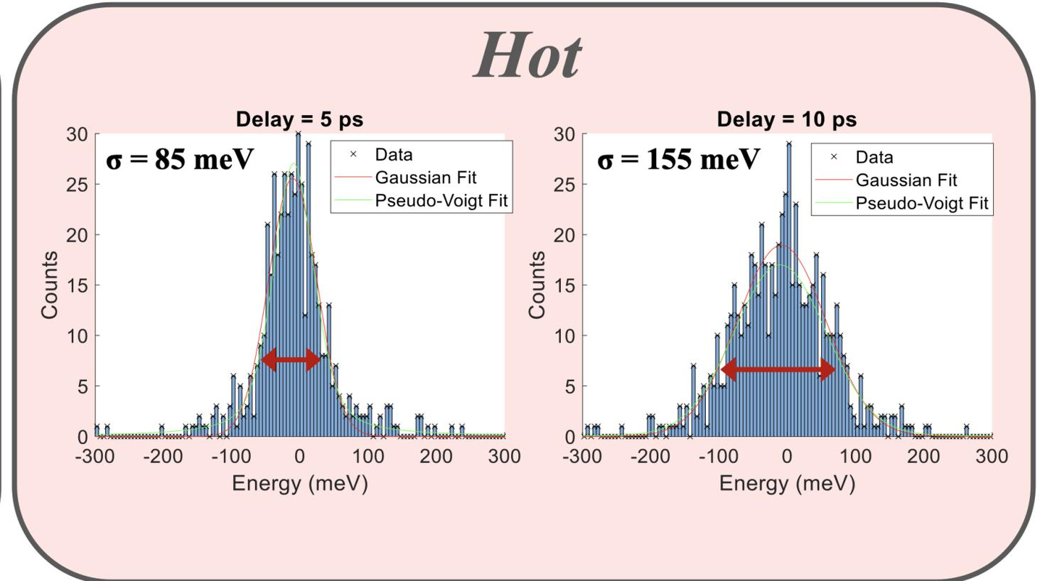
These 'hot' spectra are taken at 5 ps and 10 ps after laser irradiation. The instrument function is additionally broadened by a Gaussian with a width corresponding to the velocity distribution of the ions. As the target was destroyed on each shot, the shot rate for these spectra was 1 Hz and Each spectrum contains around 500 photons.
