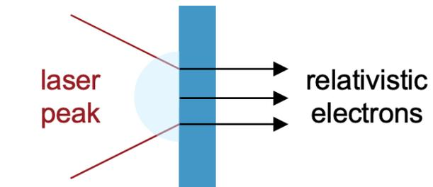
At peak intensity, electrons of this pre-plasma are accelerated to relativistic energies into the over-dense target.
