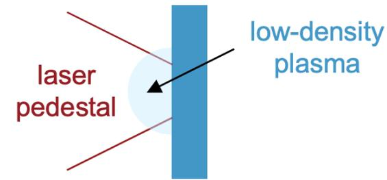
Above  $10^{18}$  W/cm<sup>2</sup>, the pedestal of the laser pulse creates a low-density plasma at the interaction surface.
