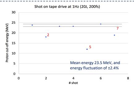
Maximum proton energy of 7 consecutive shots close obtained with the laser energy of 20J (close to maximum) and stretched laser pulse ( $\sim$ 200fs) on a Kapton ribbon 13 µm thick.
