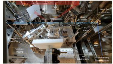
Example of 1PW setup for solid targets (TNSA)
