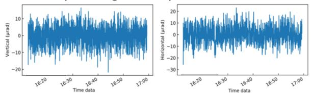
Laser pointing stability representing the laser far-field horizontal and vertical pointing fluctuation as function of time. The r.m.s. of the fluctuations is  $\pm 7$  µrad.
