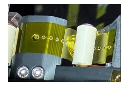
Sequence of shots on the Kapton ribbon obtained shooting with 2 J laser energy and best laser pulse compression.
