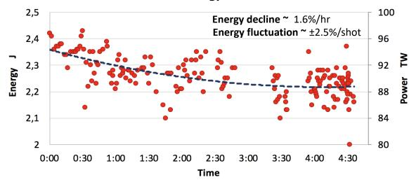
Stability of the laser pulse energy as function of time. The corresponding power is represented on the right axis.
