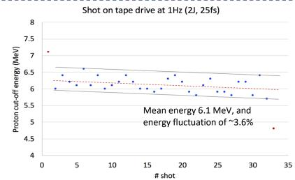
Maximum proton energy of 33 consecutive shots at low energy ( $^{\sim}2J$ ) and best compression ( $^{\sim}25fs$ ) on a Kapton ribbon 13 µm thick.
