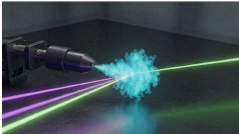
Figure 1. Illustration of gas optics operations: a pair of low-energy UV “writing beams” imprint a volume hologram in a gas to diffract a high power laser beam (shown here in green).
