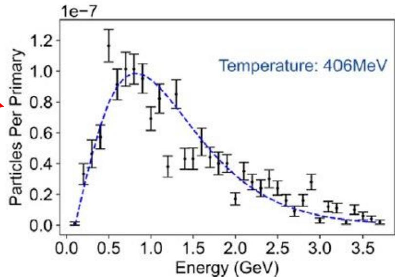
*Muon spectrum at source for a 2 cm lead target*
