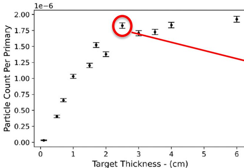
*Simulated number of muons per electron for a 5 GeV primary electron beam as a function of converter thickness. For a 1 nC electron beam, this corresponds to  $>10^4$  muons per laser shot*
