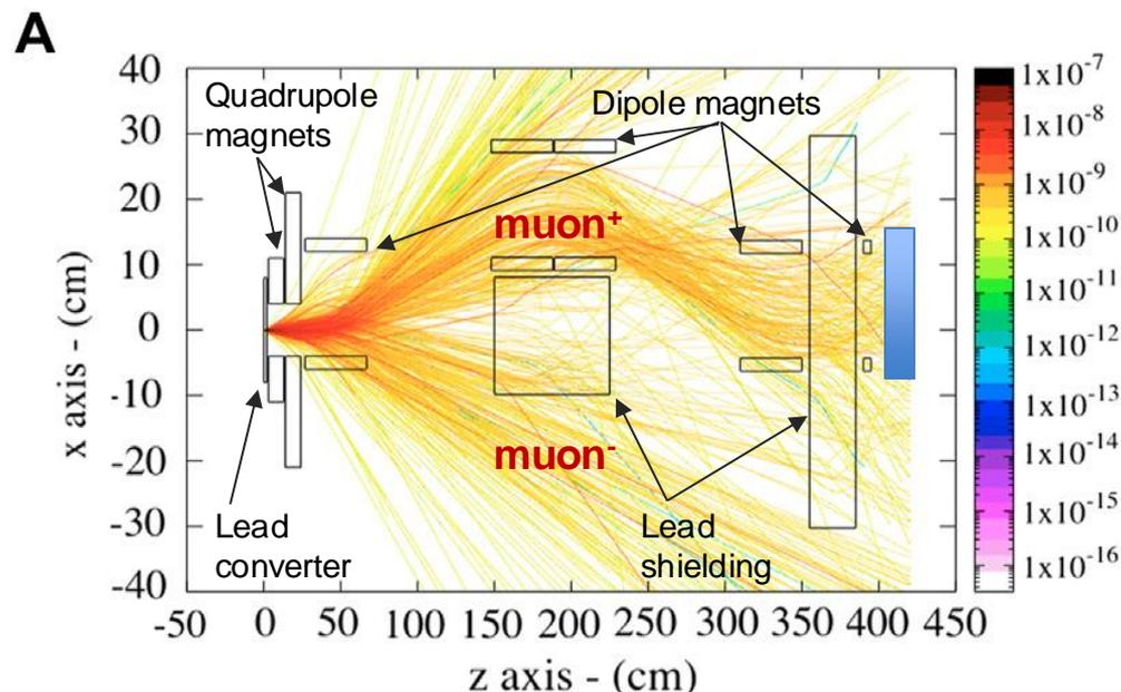
Sideview of muon trajectories through a beamline designed to provide wide-area radiographic capabilities (region for radiography highlighted in blue).
