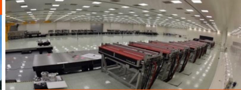
2 x 10 PW + 1 x 1 PW Laser Beam Transport System
