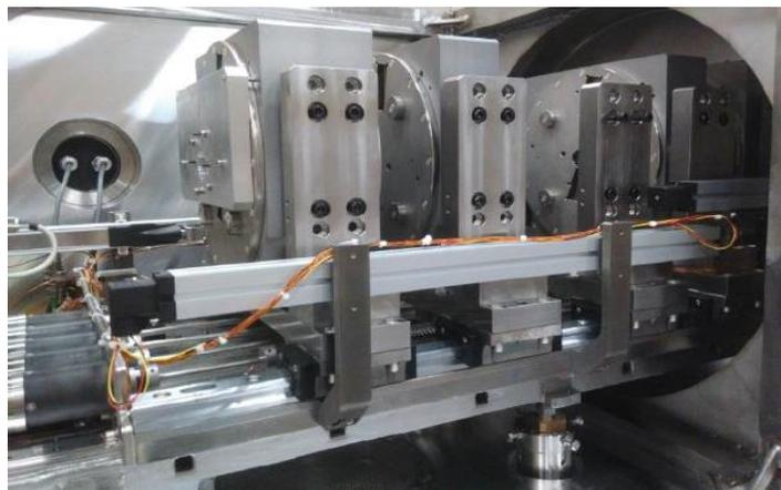
**Ion beam collimation system:**
