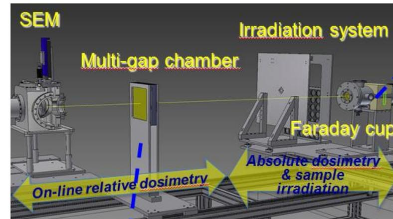
**Dosimetry and Irradiation system (in-air):**
