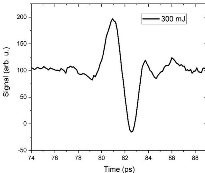
waveform of high-energy THz pulses measured by electro-optic sampling
