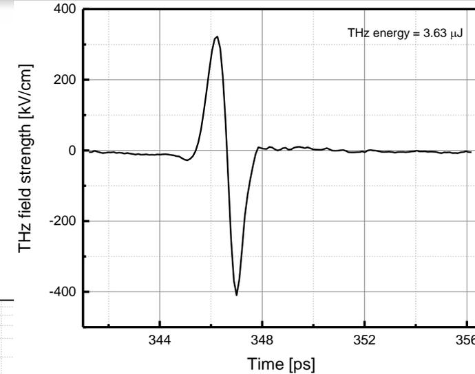
Electric field waveform and amplitude spectrum of the pump THz source (from ongoing recommissioning after facility relocation). The peak electric field strength is  $> 400 \text{ kV/cm}$ .
