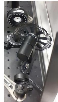
White light (probe beam) generation with sapphire plate
