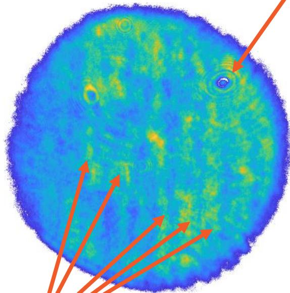
Damage of deformable mirror in TWIN 2
