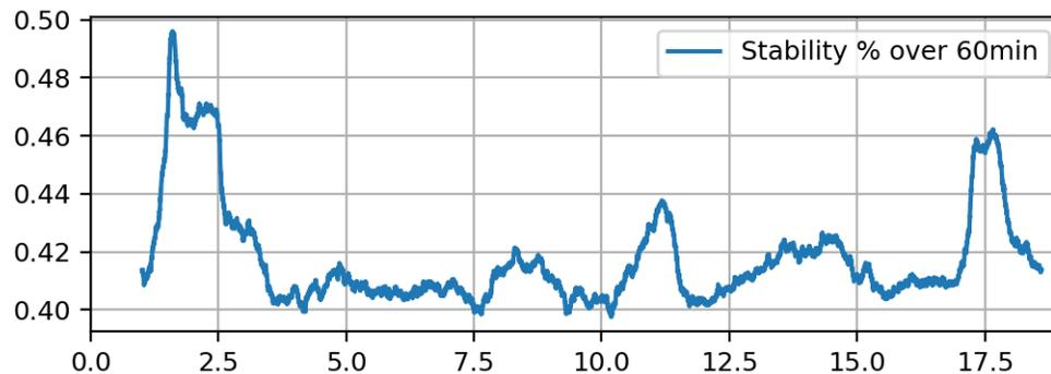
Output energy stability of the front-end over 60 min
