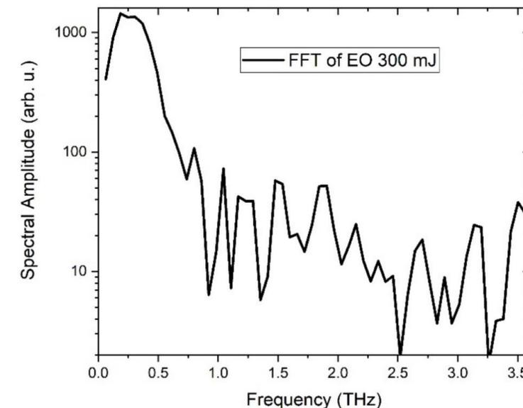
amplitude spectrum obtained by Fourier transformation of the waveform
