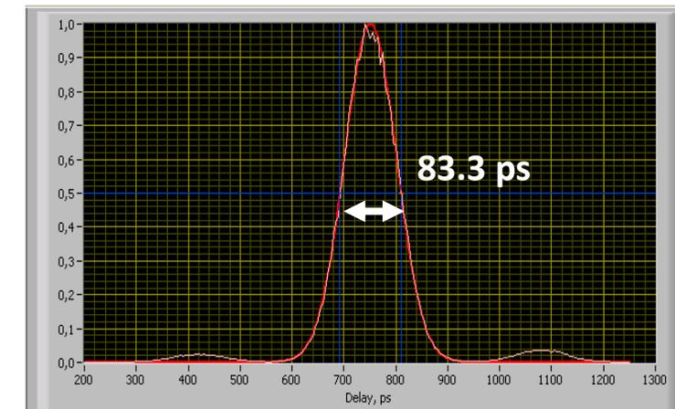
Measured typical pulse duration of PPL
