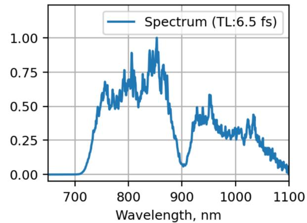
Measured output spectrum of the front-end
