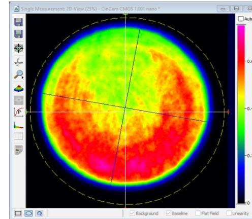
Measured typical beam profile of PPL
